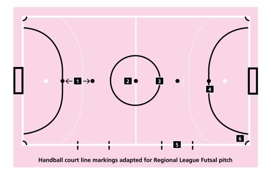
The diagram above illustrates that the additional line markings required are the penalty marks (1), centre spot (2), centre circle (3), penalty area (4), substitute marks (5) and corners arcs (6).
